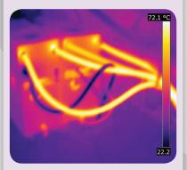
Energy losses from mold temperature controller piping can be considerable
