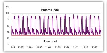
For **all-electric and hybrid** machines, the base load is much lower as motors are only running when required. Typical base loads are in the region of 10-20% and are largely accounted for by barrel heating.
