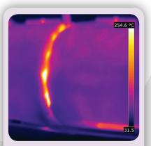
Infrared images show how barrel insulation can reduce energy losses. It will also improve operator safety
